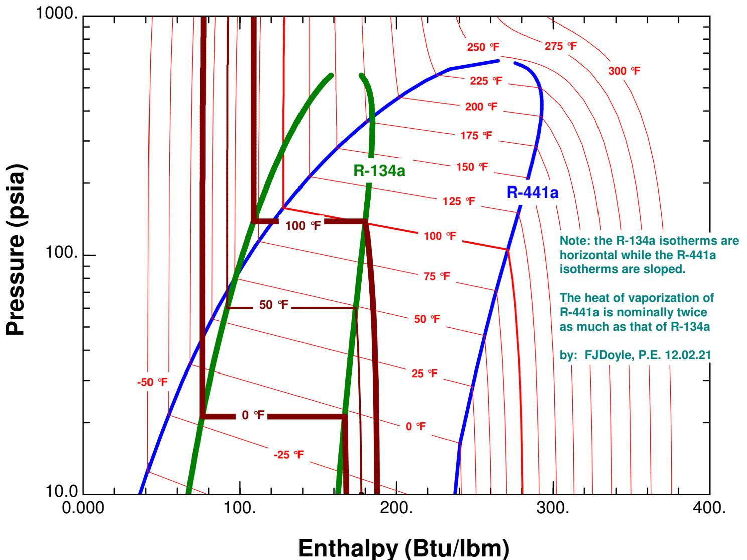
This plot shows and compares the pressure, enthalpy and temperature of R-134a and R-441a. The saturation lines for R-134a are "dull green" (wider), R-441a are "blue". The isothermal lines for R-134a are "dull red" (wider), R-441a are "bright red". From thermodynamic definitions R-134a is a "pure fluid" and R-441a is a "zeotropic" fluid mixture.
